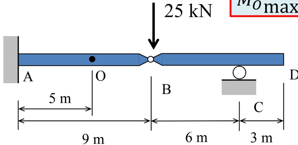
$$M_{O_{\max}}^{+} = (25 \text{ kN})(2 \text{ m}) = 50 \text{ kN}\cdot\text{m}$$
