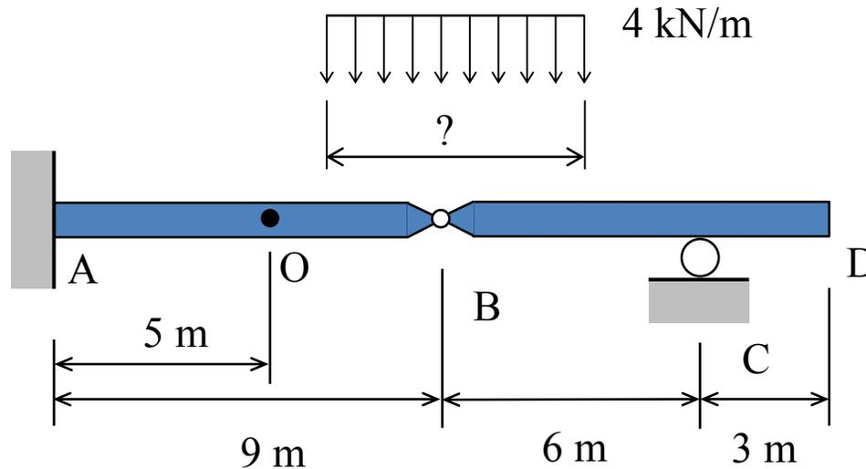
Where should we place the 4 kN/m distributed load to produce the:
