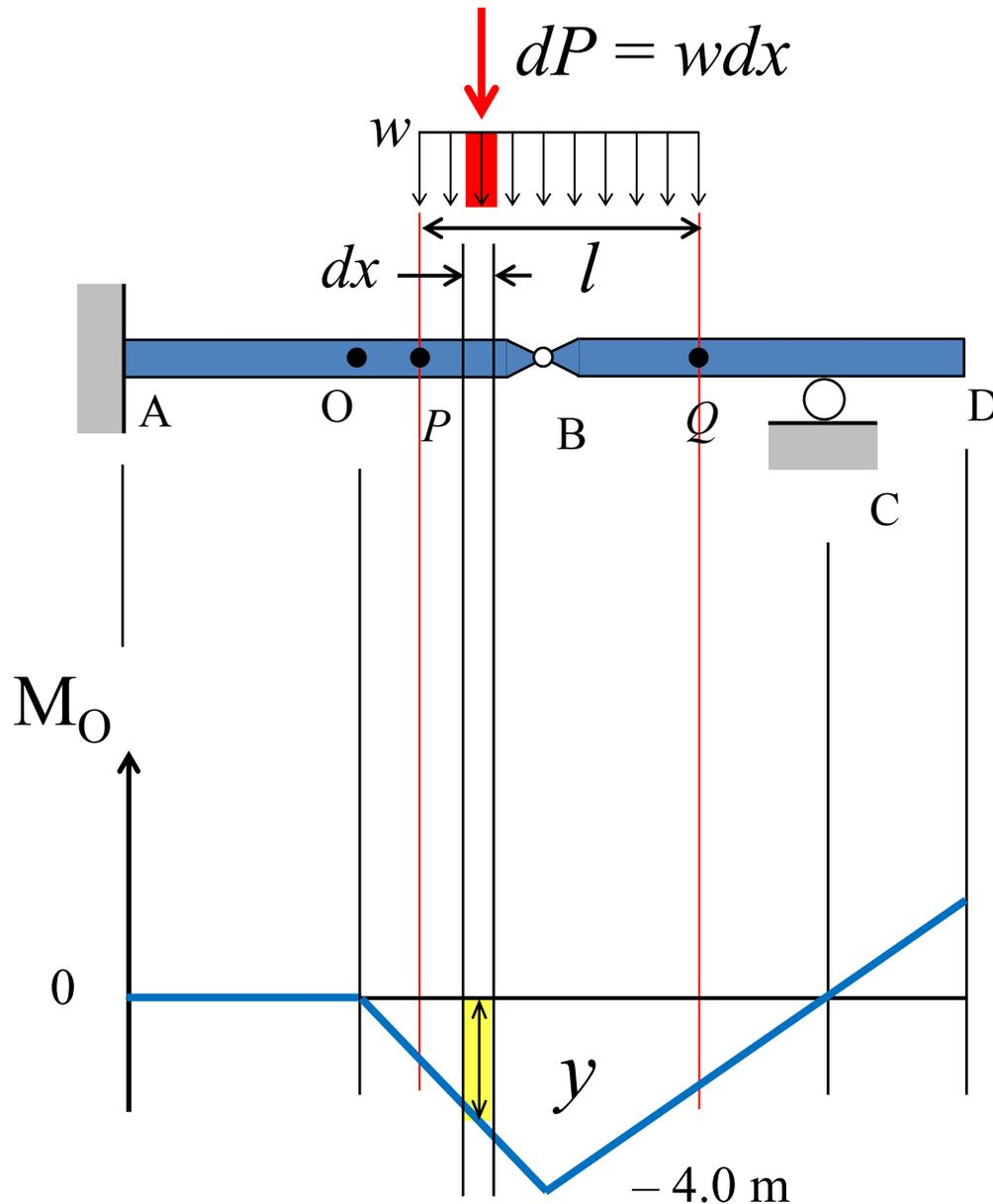
Consider a uniformly distributed load,  $w$ , acting over a length,  $l$ , between points  $P$  and  $Q$ .
