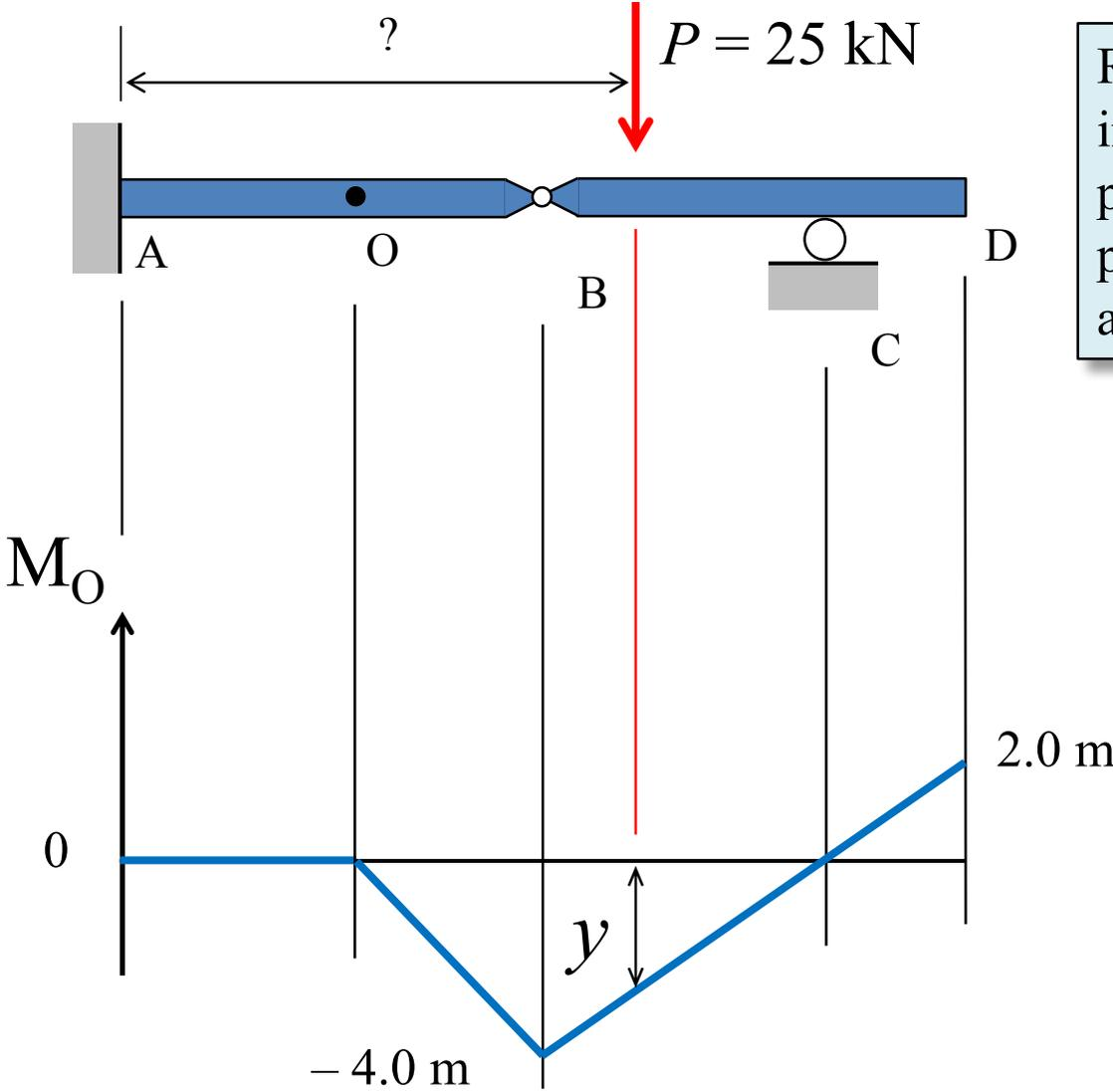
Recall that we constructed the influence line for  $M_O$  by placing a unit, dimensionless point load across the structure and keeping track of  $M_O$ .
